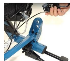
Adjustment of 30 mm changing the wheel position
