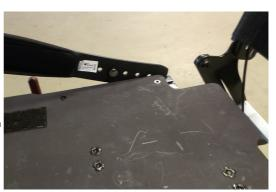
With the belt fixed to the rail on the seat plate the seat plate can swing up and follow the user when he/she is stretching.
