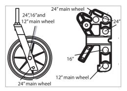
$(\mathbf{i})$ When the seat height is changed ensure that the front castors are positioned so that the front castors bearing houses stands vertical to the ground. This is vital to have good wheelchair driving characteristic.
