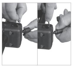
To adjust in depth, the calf pad is removed from the bracket by using an open-end spanner between the pad and the bracket. Find the required position and refix it.
