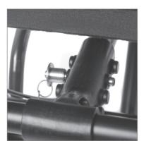
The backrest hinge has 4 holes. The hole positions are in accordance with the holes in the plastic bracket. If the locking head of the gas spring is mounted in the inner hole of the plastic bracket, the backrest hinge should also be mounted in the inner hole etc.
