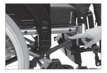
• To reposition the brake, loosen the two screws on the inside of the brake clamp.
