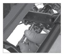
i) To check that the backrest is locked, grip the push bow and press the backrest forward. If the backrest falls forward repeat the locking procedure or contact your local dealer.
