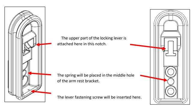
In the following 2 pictures you can see where the locking lever is inserted into the armrest bracket and where the spring as well as the lever fastening screw is placed.
