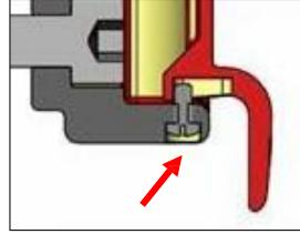
In the lever there is a long hole, which allows a movement of the lever to lock the armrest automatically after insertion.
