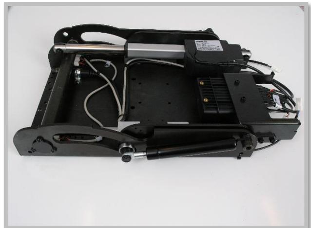
The following cables has been extended to the end of the tilt. Adding and changing part will be at the plugs at the tilt and not at the ISM module
