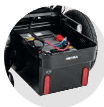
Easy battery maintenance thanks to pull-out battery case
