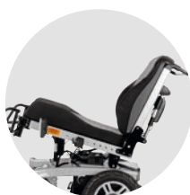
Electric seat tilt 0° to +18°
