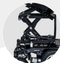
Electric seat tilt with optional 300 mm scissor lift
