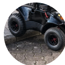
Obstacle climbing ability up to 110 mm
