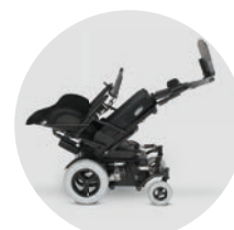
Electrical seat angle adjustment 45°
