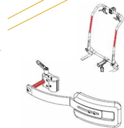
As soon as the user of the wheelchair sits in the wheelchair, position the side support in the desired height and width.
