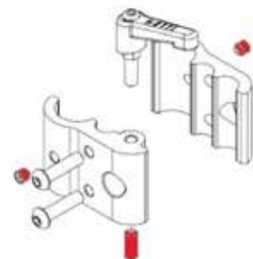
**i** The position of the clamp can be secured with the 2 at the front of the clamp additional grub screws.
