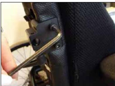
Insert the side support horizontal rod into the fixing bracket. Fix the side support cushion as far inward as desired. It is easily adjusted by loosening the Italian grip and slide the cushion in- or outward.
