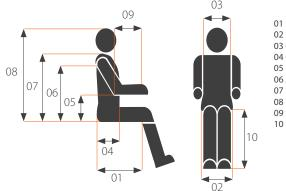
01 Seat depth 02 Seat width 03 Chest width 04 Chest depth 05 Elbow height 06 Arm pit height 07 Back height 08 Head height 09 Forearm length 10 Lower leg length
