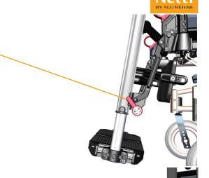
It will stay in this position and you are free to swing the leg support to required angle before you push the lock and it clicks into firmly held position.
