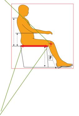
The seat depth can be adjusted. Chair-back hinge can be repositioned to adjust seat depth backwards. Extension pieces allow for increasing the seat depth in the front. Consider the wheelchair balance. See further information to seat depth adjustment on the next page and in wheelchair user manuals.
