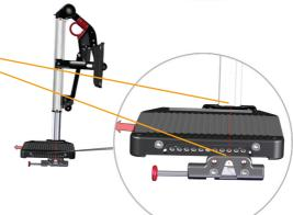
Dependent on where the lock is mounted, the lock pin must be adjusted in the length. The front button of the pin shall be positioned just behind the foot plate front.
