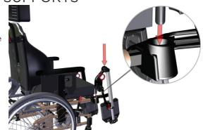
Remove the leg support by gripping through the round red release lock handle and lift the leg support straight up.
