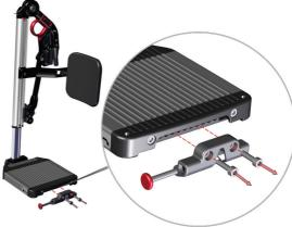
The centre of the lock must be aligned with the centre line here marked red dotted.
