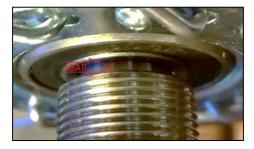
If the wheel (axle) can be moved, use a 11 open-end spanner and a 19 open-end spanner to adjust the axle play.
