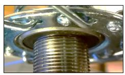
Incorrect adjustment of QR-Axle - gap between bushing and wheel axle bearing
