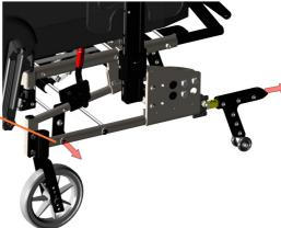
• Insert the long spring 26056 and fix it in the front.
