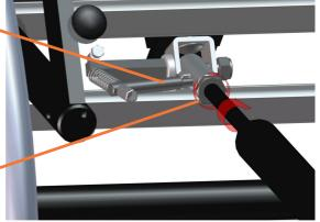
Connect the gas cylinder locking head to the plastic bracket - reconnect the quick release bolt.
