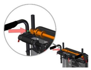
Fix the rolls at the H-bar tube in desired width. Use Allen key to fix the set screw coming with the roll.
