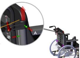
Insert the z-bars (44916 and 44917) one after the other, into the back tubes.
