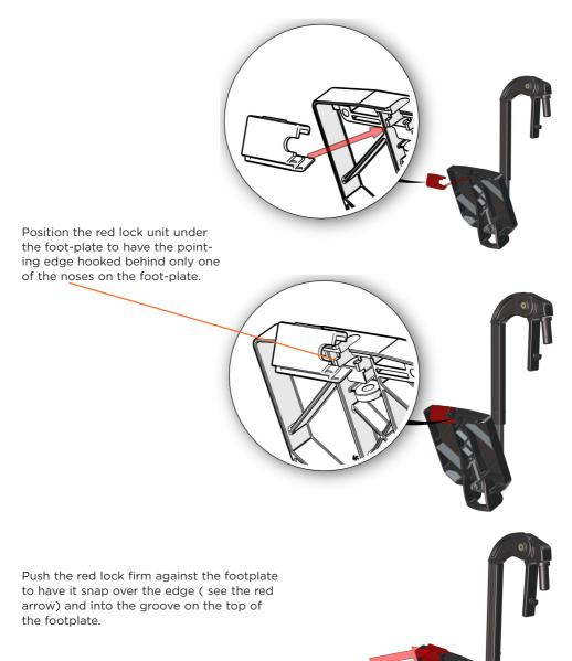
This may require a firm blow. The lock-unit is flexible and become more flexibel by warming up - for instance with warm water. It will require less effort to have the lockunit snap over the edge when it is warm.
