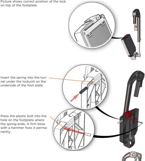
Pull the lock a couple of times to controle that it snaps back into lock position.
