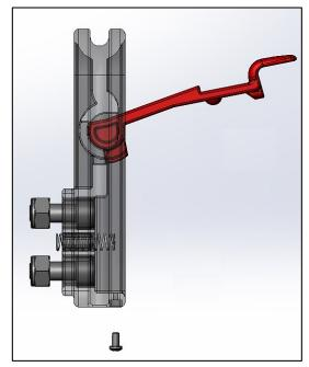
Start the mounting by placing the locking lever horizontally against the armrest bracket and slide it into the recess provided in the bracket for this purpose. Then fold the lever down.
