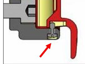
In the lever there is a long hole, which allows a movement of the lever to lock the armrest automatically after insertion.
