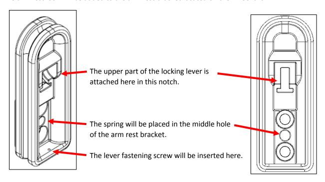
In the following 2 pictures you can see where the locking lever is inserted into the armrest bracket and where the spring as well as the lever fastening screw is placed.
