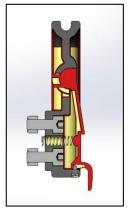
Raise the lever so far that you can insert the spring into the centre hole of the armrest bracket. Then, move the lever down again, making sure that the little buckle at the backside of the lever will meet the spring right in the middle. This will keep the spring in position.
