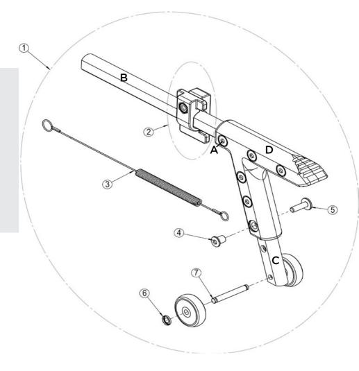
The long anti-tip spring (3) is installed in the lower wheelchair frame tube of Netti III.
