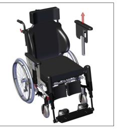
Remove the 3 rivets holding the standard cloth protector plate.
