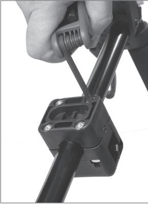
The head support bracket is fixed by tightening the four screws two by two diagonally so the bracket is fixed with the same strength divided on the four screws.
