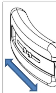
If you need to adjust the side support in height, untighten the 2 screws at the clamp, find the new position and tighten them again.
