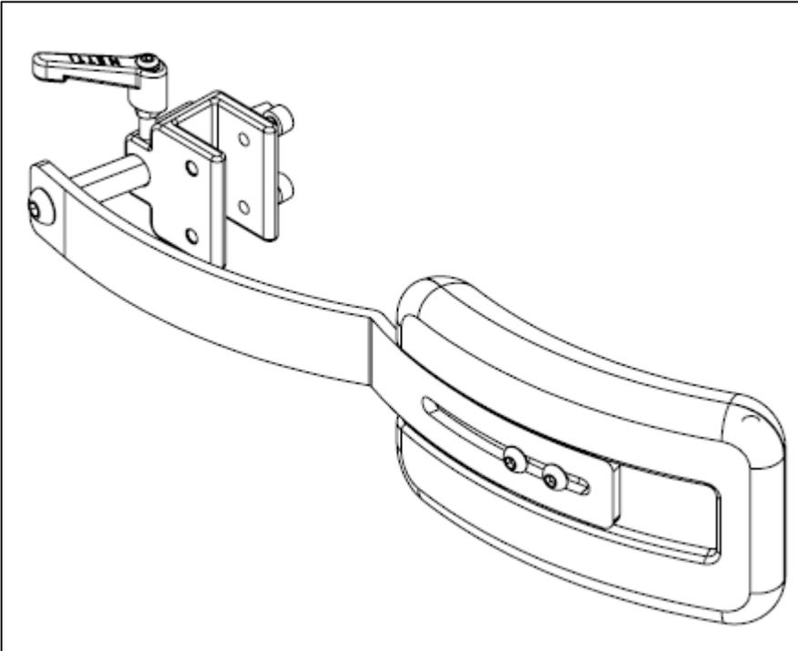
This side support can be adjusted in height, depth and side wards.
