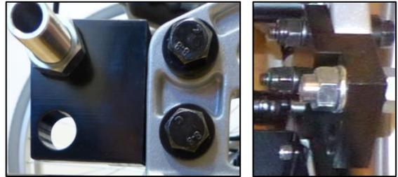
Frame and extenders should be mounted in a line.
