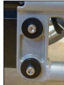
3. Finally add the extra-long antitippers (Pos. 3) to the frame and test if you can swing the antitippers upwards.
