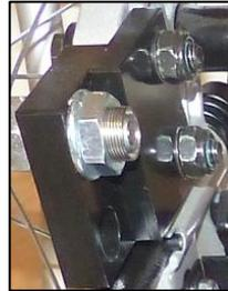
Add the wheel bushings to the extender on both sides in the needed height position.
