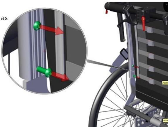
Fix the belt bracket with 2 x 2 M6x20mm hex nut screws delivered together with the brackets.
