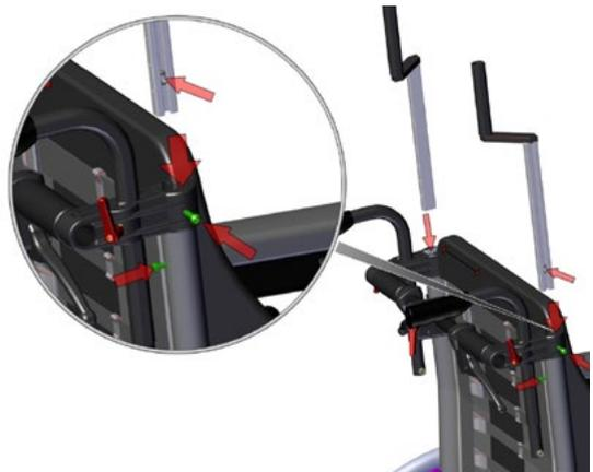
The H-Harness attachment brackets for **Netti Mini** has z-brackets with 3 holes in the upper vertical part.
