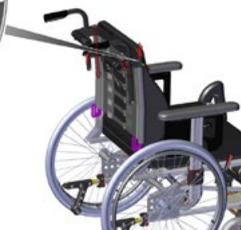
Insert the z-bars (44916 and 44917) one after the other, into the back tubes.
