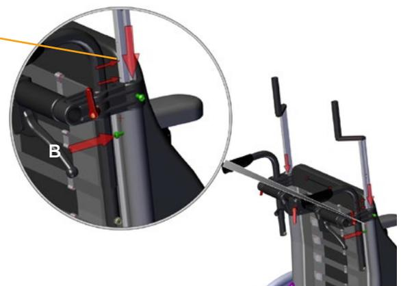
Insert H-belt bar to no. 25949 or no.25441 - to the z-bars.
