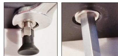
Now check if the locking ball falls smoothly into the slot of the bracket and adjust locking pin or setscrew if needed.
