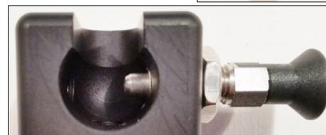
A too far in screwed thread will prevent the locking ball from falling completely into the slot.
