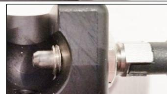
With Allen key 5 screw the setscrew in the opposite hole of the bracket. Later on you can adjust the locking tension with this.
