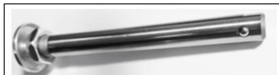
When you release the push button, the balls will stay out of the axle and will fix the axle in the wheel bushing.
