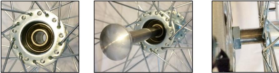
How far a wheel bushing is mounted outwards depends on if you have a chair with or without a seat width extension kit. With an extension kit the bushing will have a bigger distance to the frame.
