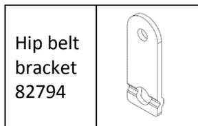
To add the hip belt bracket to the dynamic seat plate, add the square nut 20296 to the rail of the seat plate and fix the bracket from outside with the Hexagon bolt 29089.
